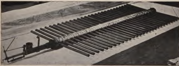
Fig. 91.—The burner employed in my steam experiments. This produced a dense and uniform blue purple flame 20 inch deep.
